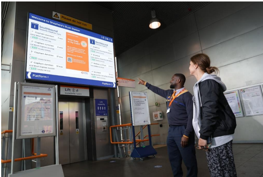
2021: Roll out of 129 upgraded customer information screens completed. The screens are installed at 35 stations and include a 4mx2.5m flagship screen at Shepherd's Bush station, which trials the busyness indicator technology. This is followed by the rollout of busyness indicator screens at 33 London Overground stations in April 2023, helping passengers to work out where to stand on the platform.
